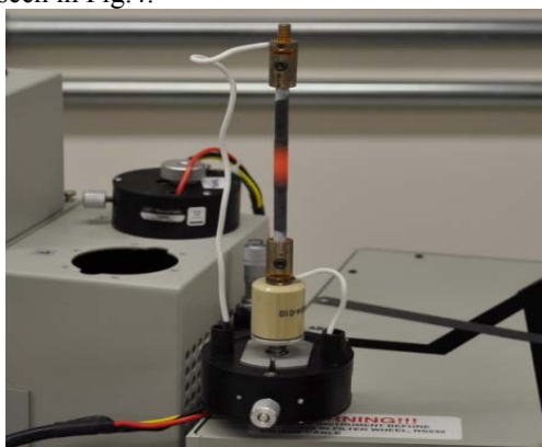
Fig. 4. Silicon Carbide element at 1075K, used as a gray body.
