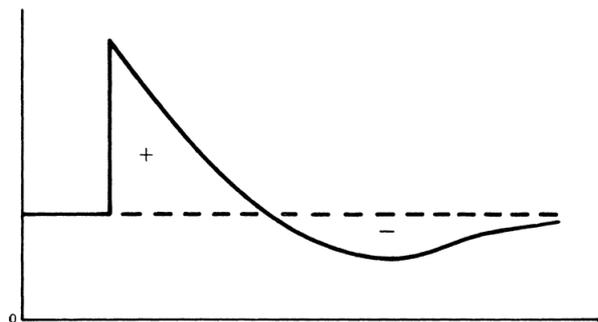
Fig. 2 - Blast wave pressure versus time
