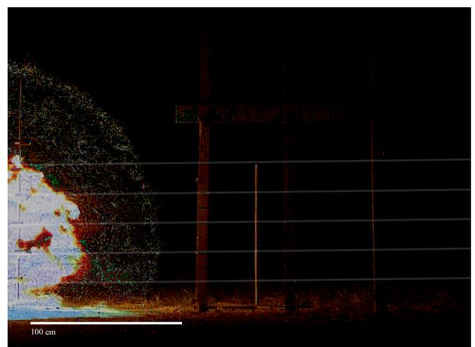
Fig. 10 - Processed video frame. Blast wave sharp and well defined.
