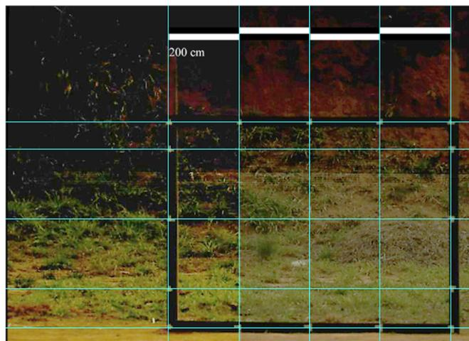
Fig. 11 - Target stickers, aligned and spaced with the assistance of a total station combining electronic theodolite and electromagnetic distance measuring instrument improve the accuracy of position measuring in the final image.
