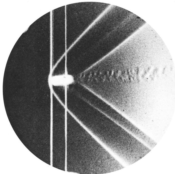
Fig. 1 - Photograph of shockwaves around a supersonic bullet, published by Ernst Mach in 1887.
