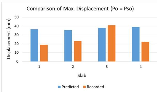
Fig. 7. Comparison of predicted and recorded maximum displacement with  $P_{so}$  as  $P_0$ .
