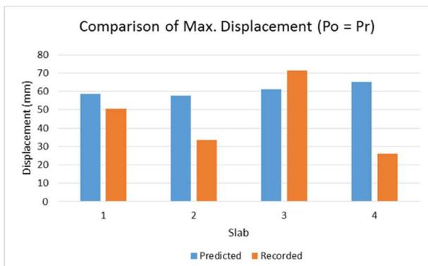
Fig. 8. Comparison of predicted and recorded maximum displacement with  $P_r$  as  $P_0$ .
