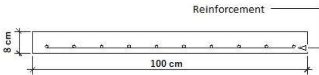
Fig. 4. Cross section of the slab.
