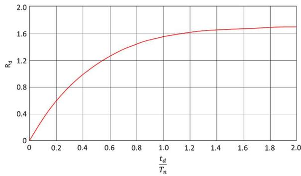
Fig. 3. Shock spectra for triangular pulse.
