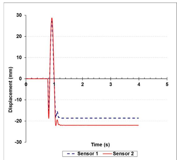
Fig. 6. Record of displacement meter of slab 1.
