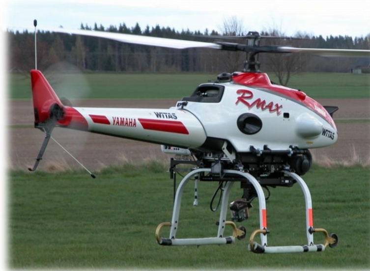
Yamaha RMAX weight 95 kg, length 3.6 m
