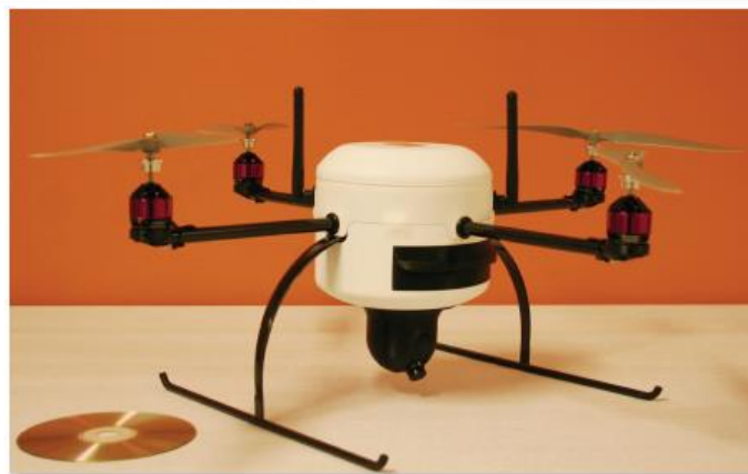
LinkQuad weight ~1 kg, diameter ~70cm
