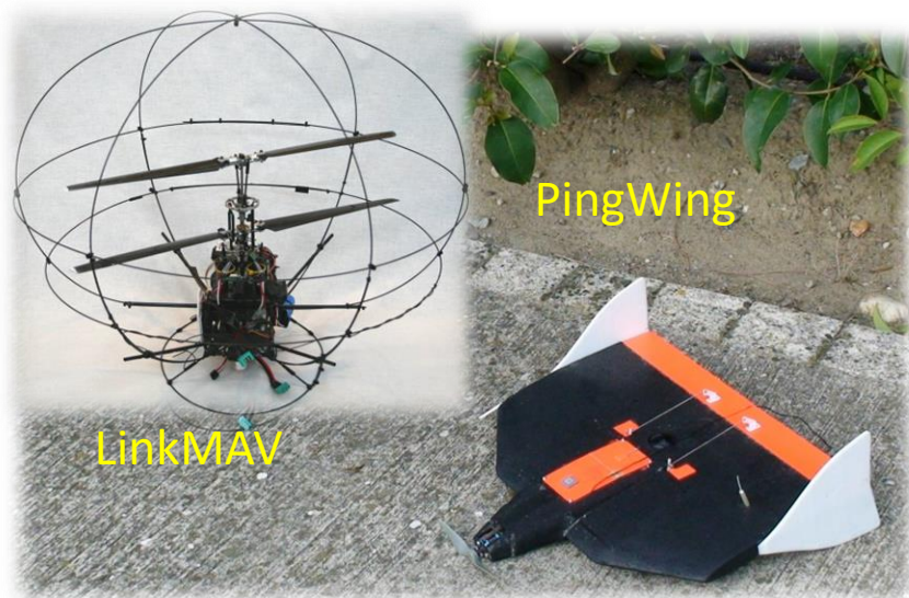
Micro UAVs weight < 500 g, diameter < 50 cm
